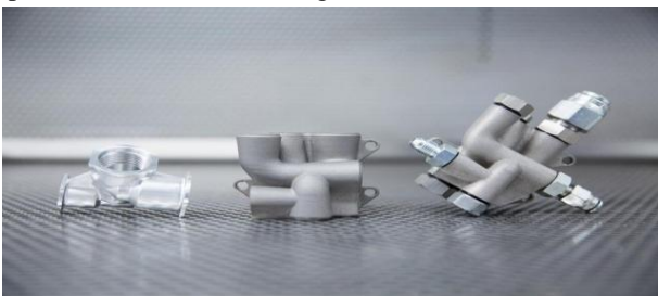
Fig.4. Manifold Weight reduced part by 60%
