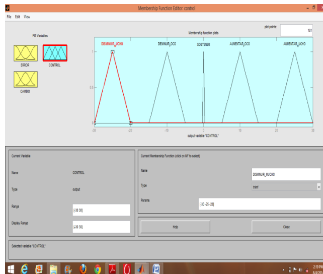
Fig. 8 Membership Functions of Output Control Torque
