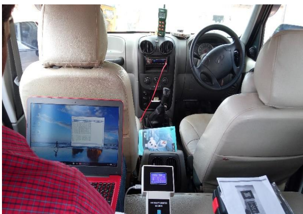
Fig. 3 IAQ Monitor with DAQ
