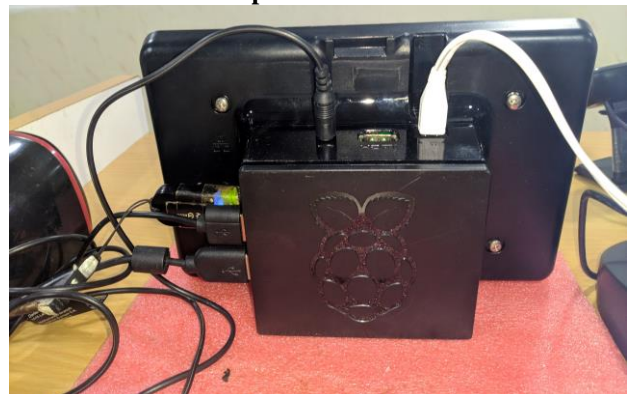
Fig. 11 LCD touch screen and main control unit placed on the podium back view
