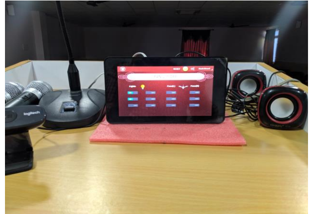
Fig. 10 LCD touch screen and main control unit placed on the podium front view
