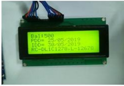
Fig. 10. Vehicle's Insurance Due Date (IDD) & Pollution DueDate(PDD) on LCD
