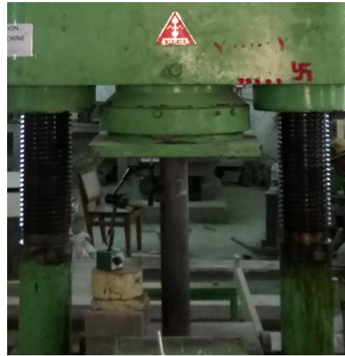
Fig. 2 Column testing setup
