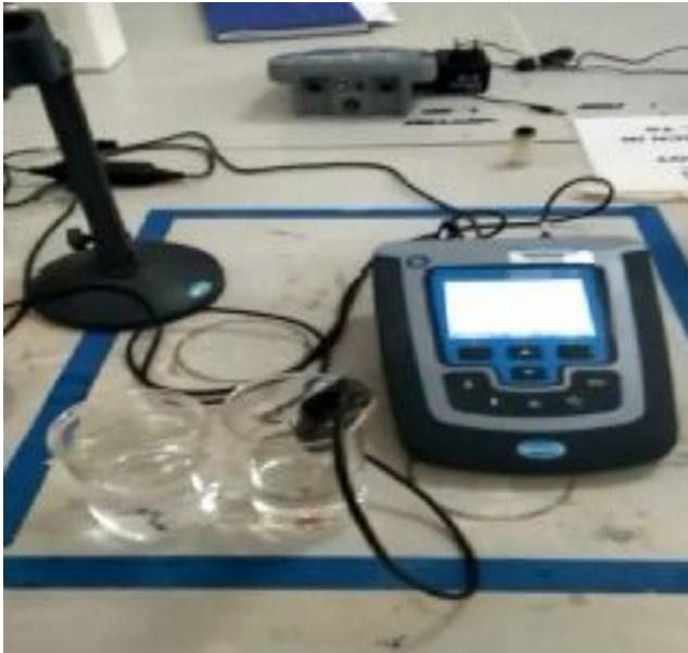
Fig. 7: Leachate collected was measured using pH meter
