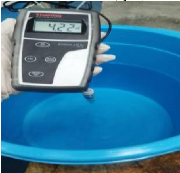
Fig. 8: Leaching fluid were measured until reached pH 4.2
