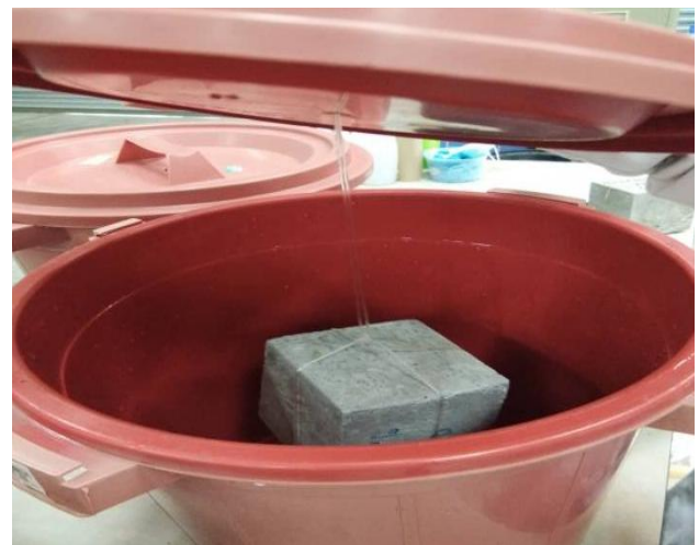
Fig. 5: S/S matrices were suspended in the leaching fluid
