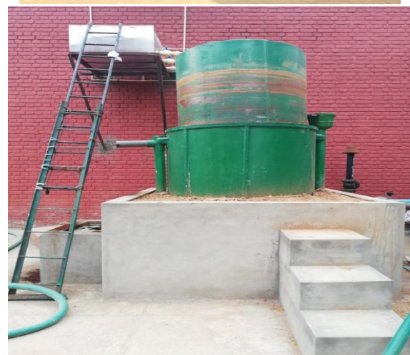
Fig 2: Pictorial outlook of the experimental unit (a) at initial stage (b) after formation of biogas
