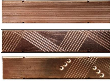
Fig. 6 Novel cannelure fin structure and its combination with dimples
