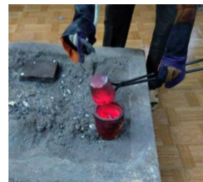
Fig. 8 - Adding of reinforcements
