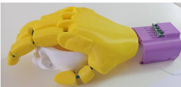
Fig. 9 Assembled Prosthetic Hand for Symbrachydactyly Patient
