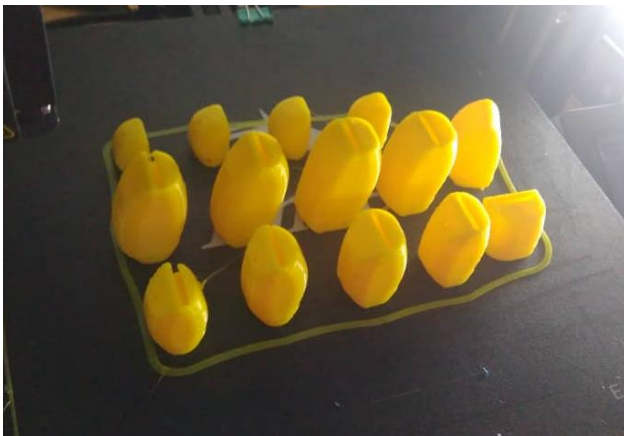
Fig. 8 Samples of the 3D Printed Part of the Prosthetic Hand
