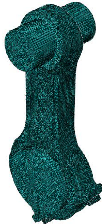
Fig. 2. Finite element model of connecting rod
