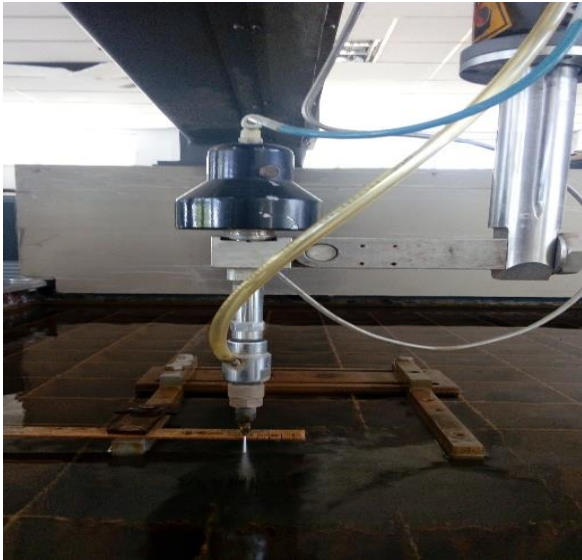
Fig. 1. Abrasive water jet machine nozzle setup
