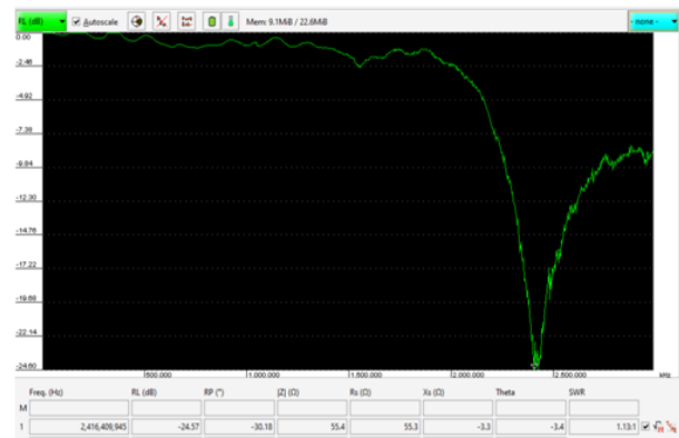
Fig. 7 The S-parameter of the fabricated antenna
