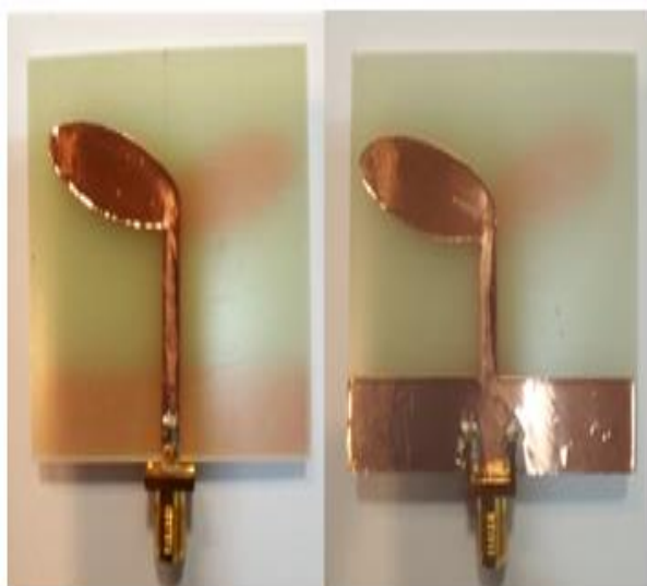
Fig. 6(a)Front vision of the prototype antenna (b)Back vision of the prototype antenna
