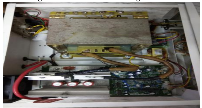
Fig.9 Hardware implementation of inverter with transformer
