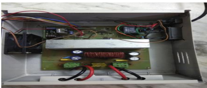
Fig.7 Hardware Implementation of MPPT with DC-DC converter
