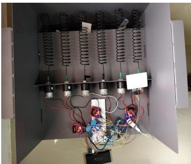
Fig.6. Project Prototype with Circuit Connections
