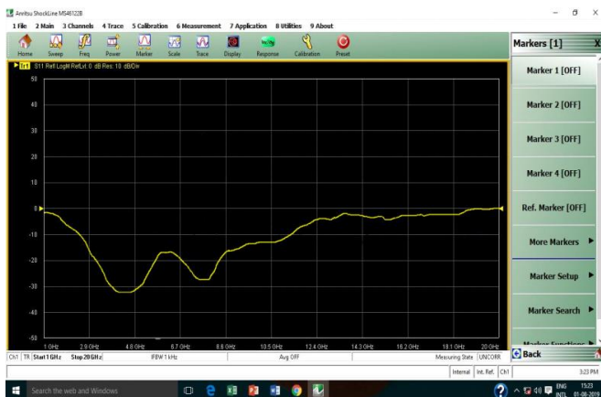
Figure 8: Shows the VSWR of Hardware of Proposed compact super wideband antenna
