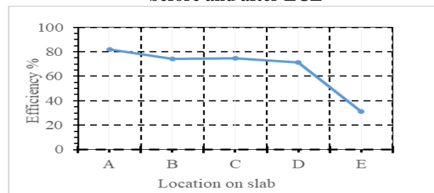
Fig. 9: Chloride extraction efficiency at different location
