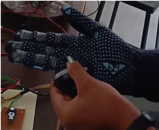
Fig.3 Working of Flex Sensor
