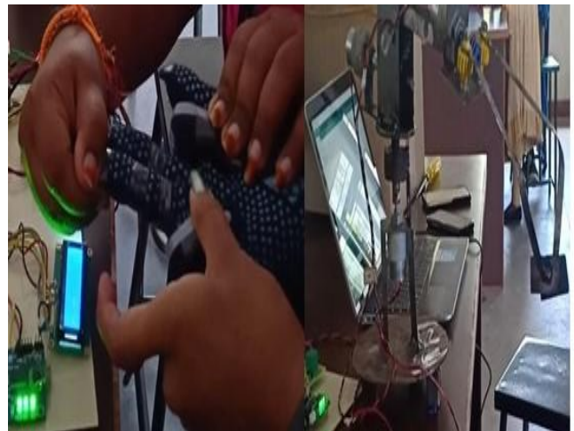
Fig.11 Flex Sensor F4 and F4 was bent, Arm moves right
