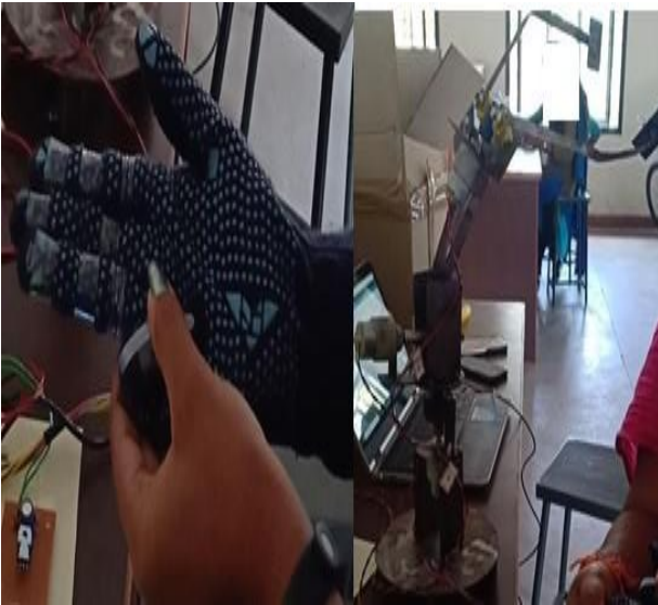
Fig.6 Flex Sensor F1 was bent, Arm Places the object
