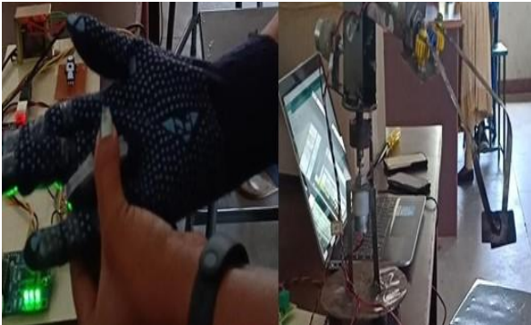
Fig.7 Flex Sensor F1 was bent, Arm moves towards left.
