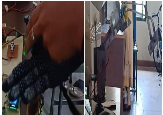
Fig.10 Flex Sensor F4 was bent, Arm picks the object.
